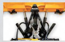
**Blade Angle Stop** Designed to transfer extreme impacts throughout the blade's structure and reduce stress on the hydraulic rams.
